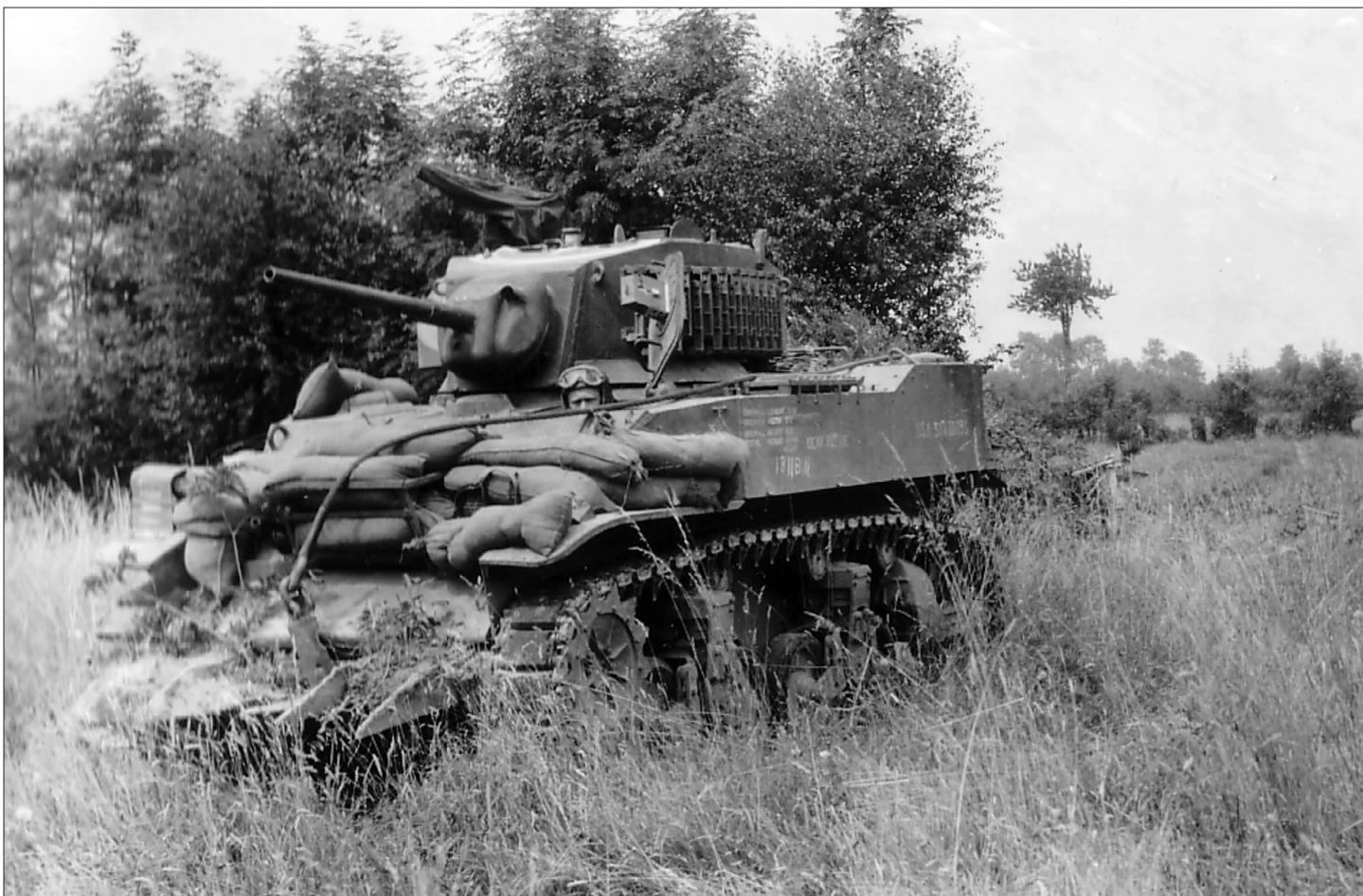
A "Rhino Tank," modified with SGT Cullin's solution to cut through the hedgerows of Eastern France during World War II. (Source: Normandy Archives)
